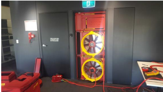
Air leakage test equipment during setup
